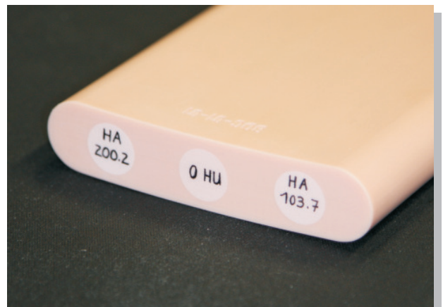
QRM-Bone in the Bone Calibration Phantom
